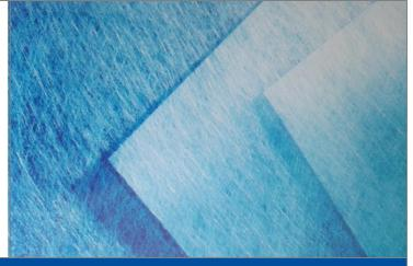
Seperator mats in battery plate separator applications
