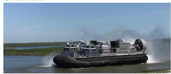
LCAC 100, Textron's first-in-class Ship-to-Shore Connector (SSC), conducts its first on-water test outside of the company's facility in Louisiana on April 10, 2018. Textron photo.
